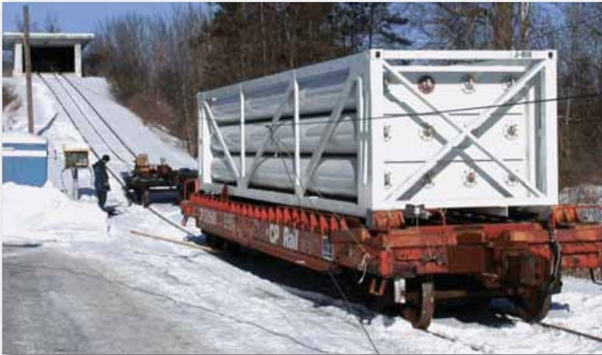
*In the impact test for a FIBA skid, the structure is rolled downhill into a concrete-filled railroad car. Cables and sensors measure structural movement.*
