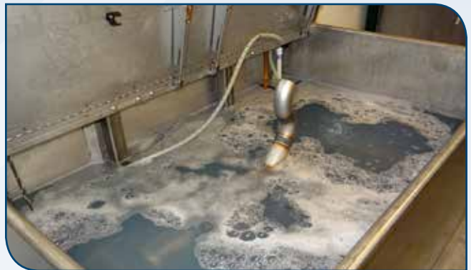
Cleaning for Oxygen Service
